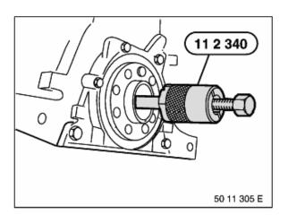
Remove thrust bearing with special tool 11 2 340 .
