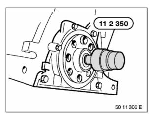
Install new thrust bearing and drive firmly home with special tool 11 2 350 in conjunction with special tool 00 5 500 .
